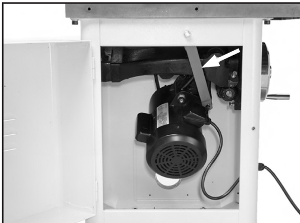
Fig.5: shipping brace location
